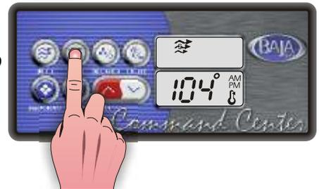
**Blower Key:** Press this key once to turn the Blower onto High speed, a second press will turn the Blower onto Low speed, a third press will turn the Blower off. A built-in timer will shut the blower off after 20 minutes of operation unless done so manually. The Blower Icon will appear while the blower is running in High speed and flash while it is in Low speed.
