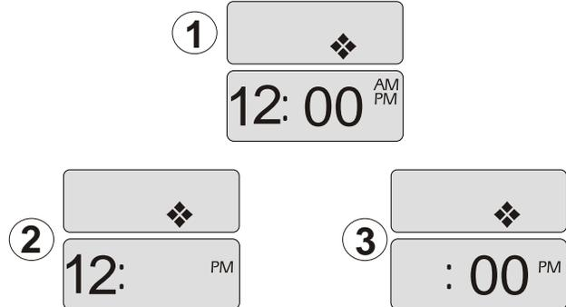
**Filtration Start Time 1: ("Fon1")** appears in the display. To adjust, **(1)** press the **Enter (Light) key**, Use the Temp. Set keys to adjust the hour from 01 to 12. **(2)** Press the **Program key** then **Enter (Light) key** to adjust minutes, use the Temp. Set keys to adjust the minutes from 00 to 59. **(3)** Press the **Program key** to confirm the new setting and move to the next parameter to be programmed.
