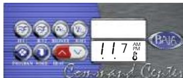
If 3 flashing below the temperature display and the temperature displayed is 115° F or higher, and over temperature condition and a need for service has occurred.
