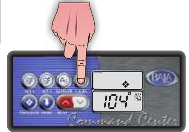
**Time of Day:** This is the first parameter and will automatically appear with the hour flashing. To adjust, **(1)** press the **Enter (Light) key**, use the Temp. Set keys to adjust the hour from 00: to 11:.. **(2)** Press the **Program key** then **Enter (Light) key** to adjust minutes, use the Temp. Set keys to adjust the minutes from :00 to :59. **(3)** Press the **Program key** to confirm the new setting and move to the next parameter to be programmed.
