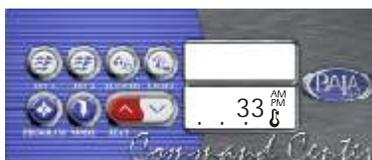
If the actual spa water temperature greatly differs from the displayed temperature or the display reads a constant 33° F, a temperature sensor error and a need for service has occurred.
