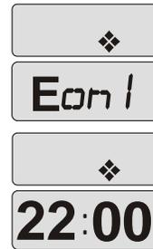
**Economy Duration 1: ("Edu1")** appears in the display. To adjust, (1) press the Enter (Light) key. Use the Warmer/Cooler keys to adjust from OFF (always off) to 24 (always on). (2) Press the Program key to confirm the new setting. The display will then return to the next parameter to be programmed. **Factory set 8 hours (10PM-6AM)**
