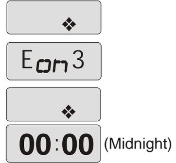
**Economy Duration 3:** ("Edu3") appears in the display. To adjust, (1) press the Enter (Light) key. Use the Warmer/Cooler keys to adjust from OFF (always off) to 24 (always on). (2) Press the Program key to confirm the new setting and exit to the Time/Temperature display.
