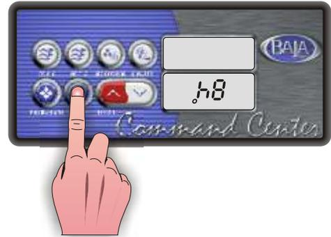
**Panel Lock:** It is possible to lock all of the spaside control keys. Press and hold the Pump 1 key for 5 seconds, "LocF" will appear indicating all the keys have been locked. To unlock keys, simply press and hold the Pump 1 key for 5 seconds until "Uloc" will appear indicating the spaside has returned to normal operation.
