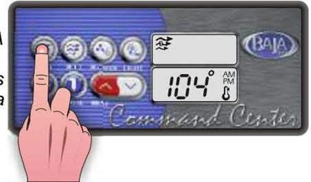
**Jet 2 Key:** Press this key once to turn Pump 2 onto High speed, a second press will turn the pump off. A built-in timer will shut the pump off after 20 minutes of operation unless done so manually. The Pump 2 Icon will appear in the upper LCD window while the pump is running in High speed (WhiteWater™ Series Only).
