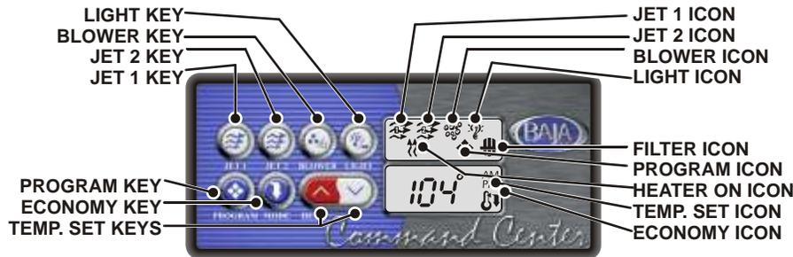
**Default System Operation:** When power is applied, or there is a temporary Loss of power, the system will initiate its default programming. The filter cycle will begin 24-hours after the system has been powered up. The filtration cycle will be Active for 1-hour and will repeat every 24-hours. The temperature will be maintained at 95°F
