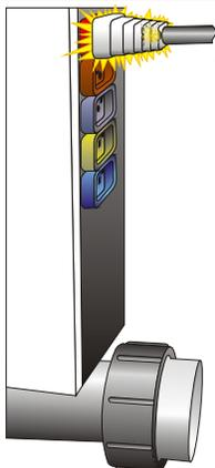
The cords that connect the vital components of your spa to the control have been equipped with internal diagnostic indicators. Whenever a component is operating, that components corresponding plug connection will illuminate to let you know that proper voltage is being supplied.
