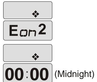
**Economy Duration 2: ("Edu2")** appears in the display. To adjust, (1) press the Enter (Light) key. Use the Warmer/Cooler keys to adjust from OFF (always off) to 24 (always on). (2) Press the Program key to confirm the new setting. The display will then return to the next parameter to be programmed.
