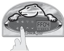
Press the filter cycle key again to display the number of cycles (FF) in a 24 hour period. You can select from 1 cycle to 4 cycles per day. The Filter Cycle triangular icon will appear on the display when a filter cycle is on.
